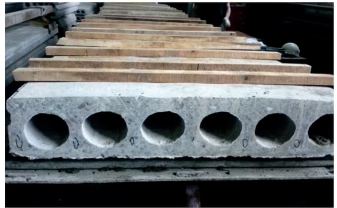
Fig. 8: End of slab with measured depth of strand slip
