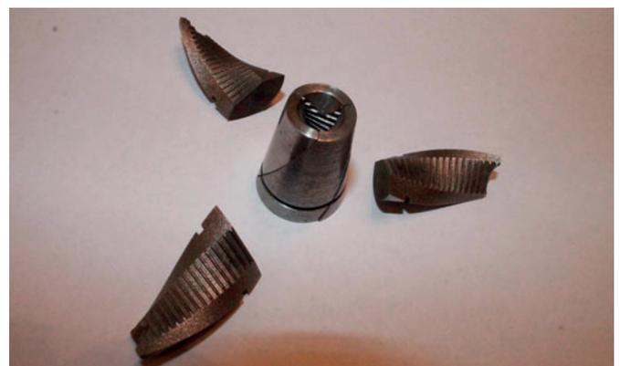
their colleagues from precast concrete plants asked to develop new configuration of anchor grip, because existing grip isn't reliable in work with the trihedral strand.
