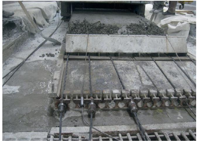
Fig. 6: Dry casting line with combined reinforcement.
