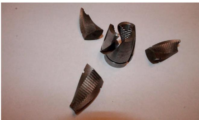
Fig. 9: 1<sup>st</sup> version of anchor grip for trihedral PC strand.
